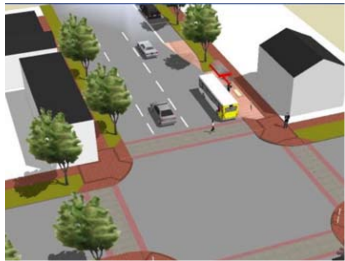
Plan and views of recommended conversion from four to three one-way lanes. The three-lane section also permits a deeper tree lawn and on-street parking.
